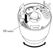
It is necessary to set a peculiar camera address, protocol, and bit rate as each camera. Please set up a camera address according to the following table.
